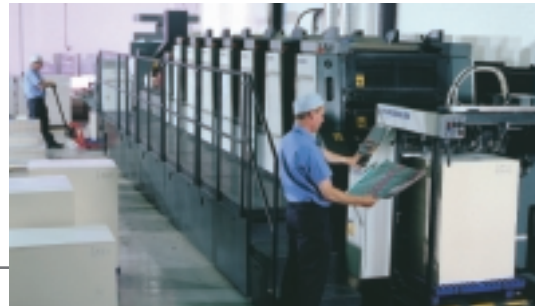
Cartons being printed on a small format multi-colour offset press in an M.Y. Cartons UK plant
