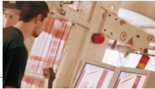
State-of-the-art AVT web scanning on Nampak Flexible's flexographic printing press
